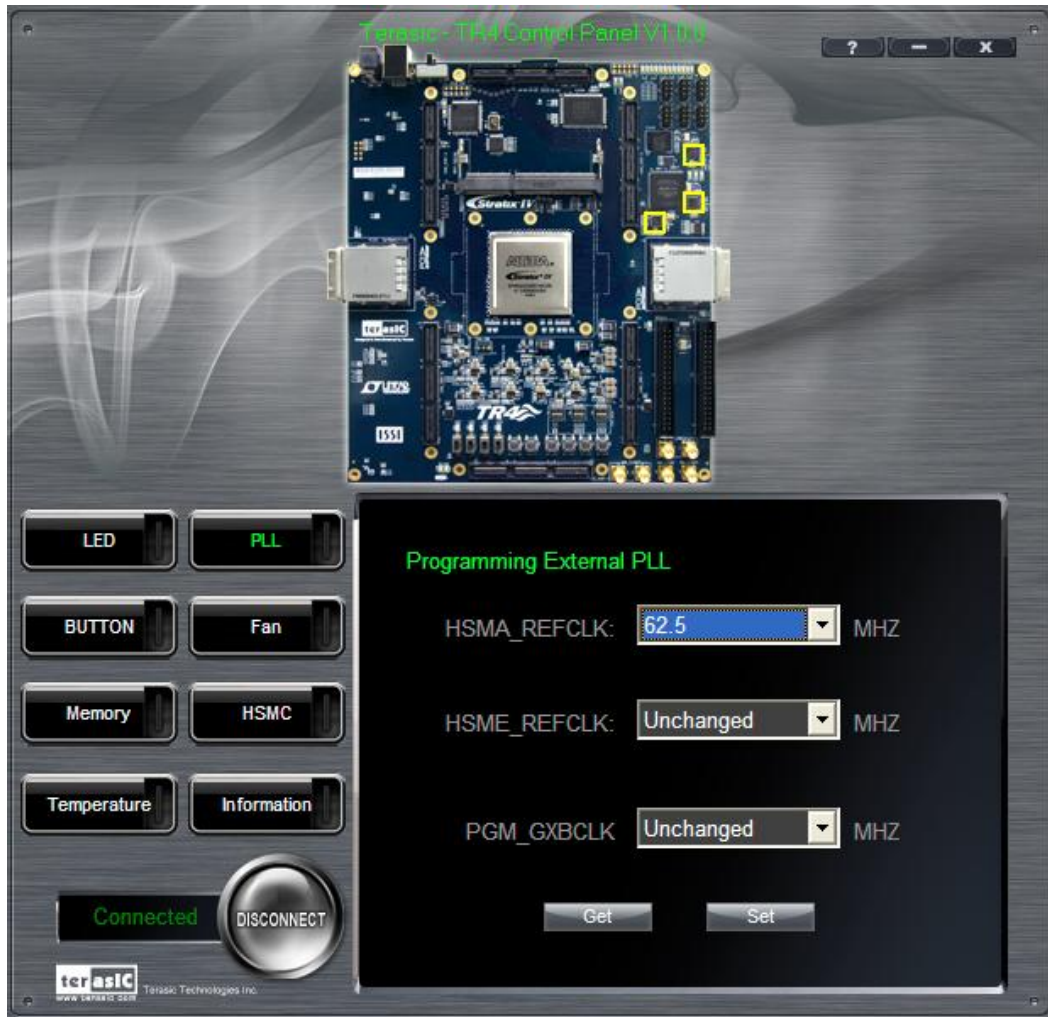
Figure 3-10 Programmable External PLL Configured through Control Panel
