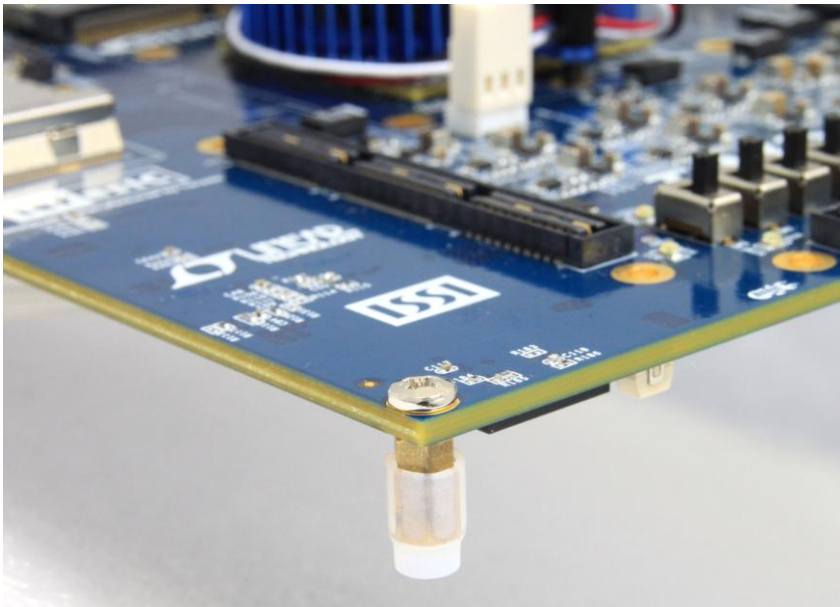
Figure 1-4 Mount Silicon Foot Stands
