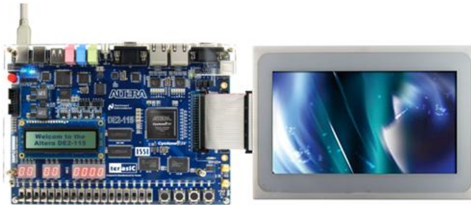
Figure 4-4 DE2-115 ePhoto Configuration Setup
