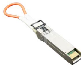
Figure 8-1 Optical SFP+ Loopback Fixture
