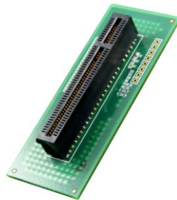
Figure 8-3 PCIe Loopback Fixture
