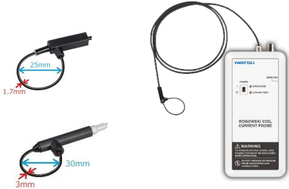
Figure 16. Rogowski Current Probe Suitable Loop Size
