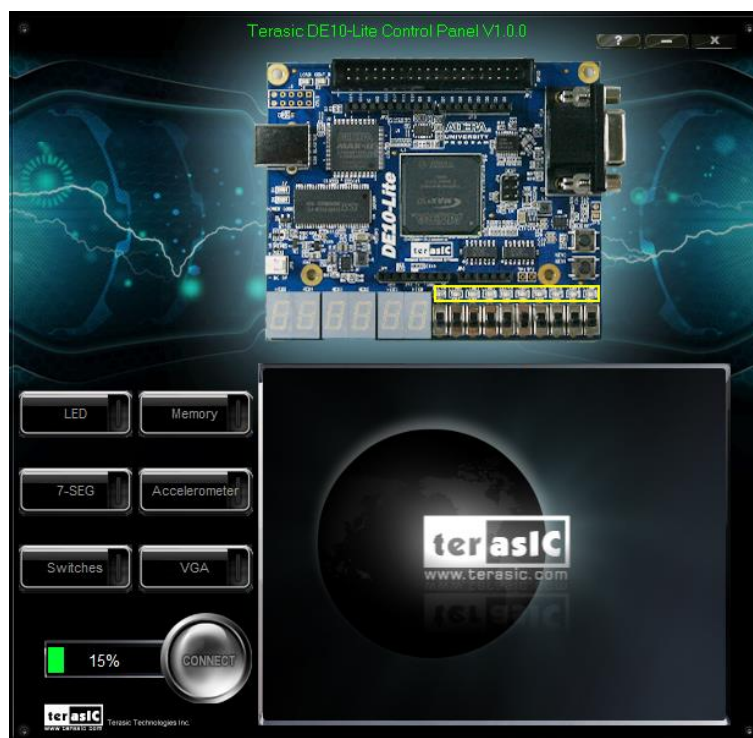
Figure 2-1 The DE10-Lite Control Panel
