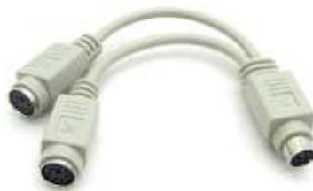
Figure 3-30 Y-Cable for using keyboard and mouse simultaneously
