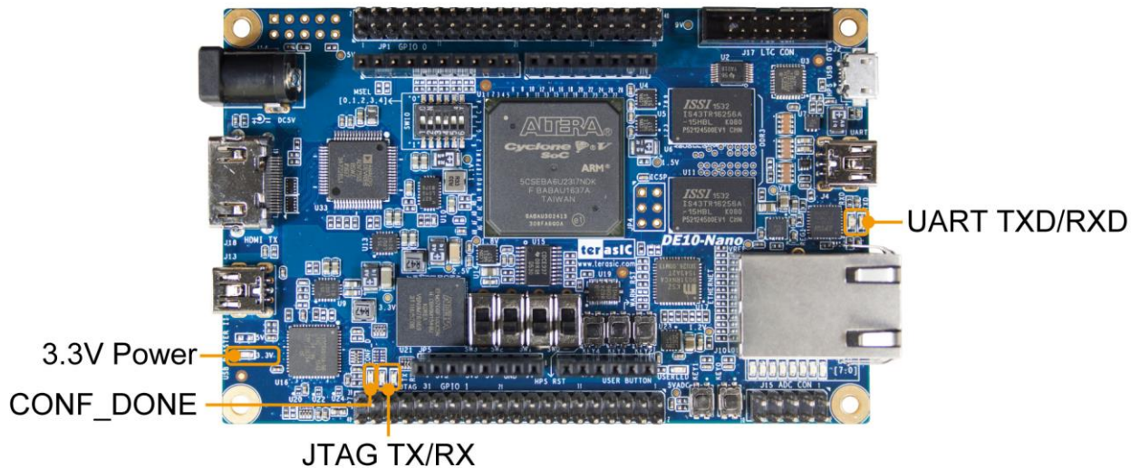
Figure 3-12 LED Indicators on DE10-Nano
