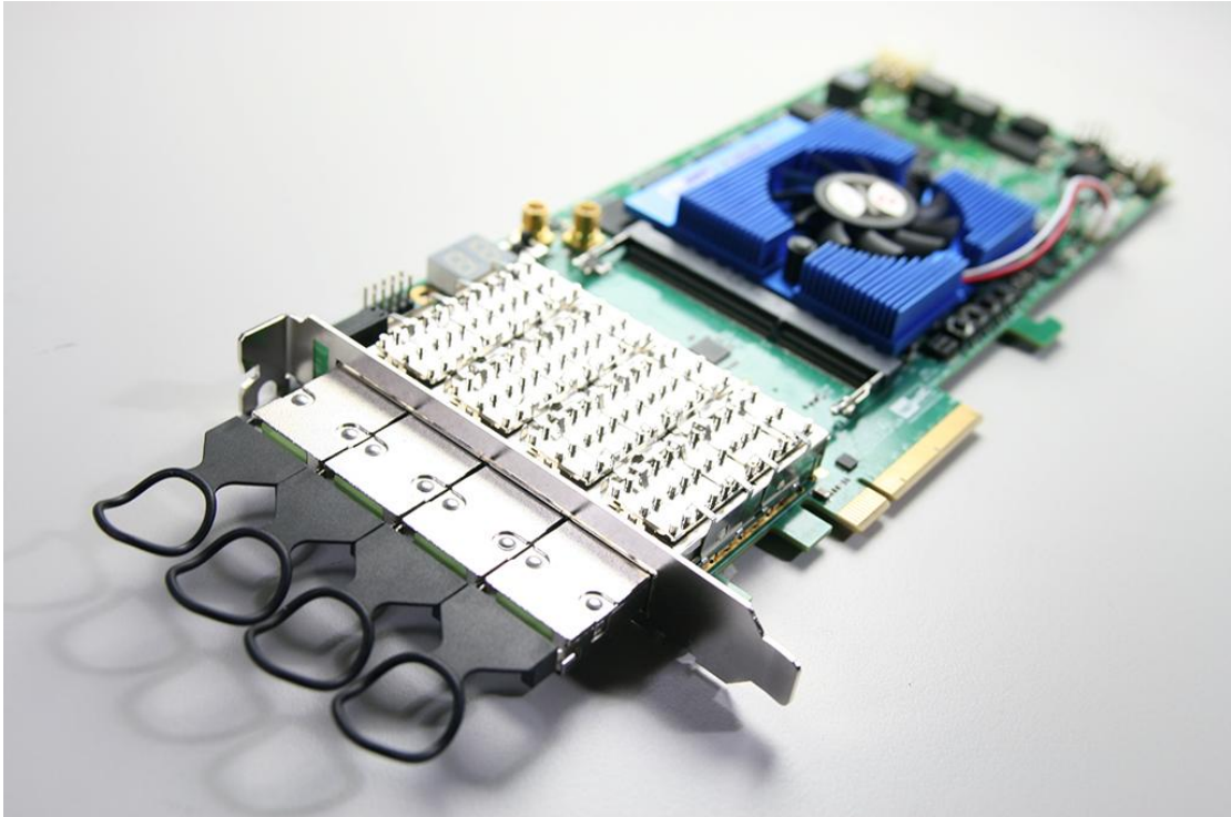
Figure 8-4 Four QSFP+ Loopback Fixtures Installed
