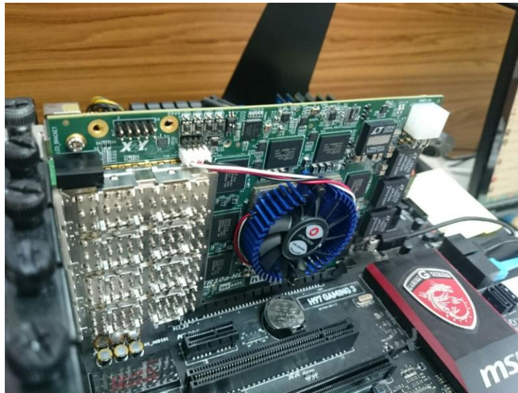
Figure 7-9 FPGA board installation on PC
