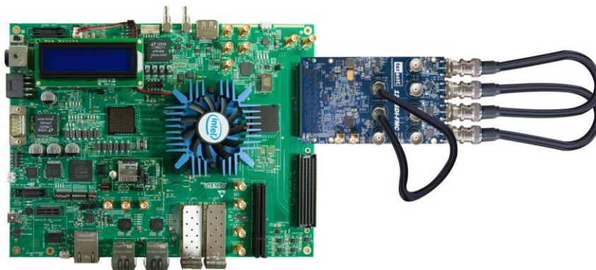
Figure 4-5 Hardware setup of SDI-FMC with A10SoC
