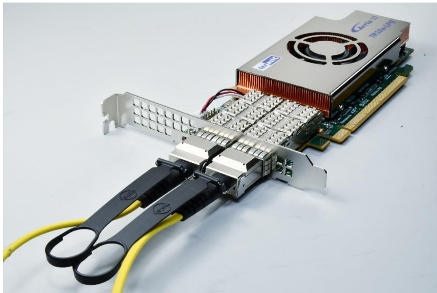
Figure 7-3 One QSFP+ Cables Installed
