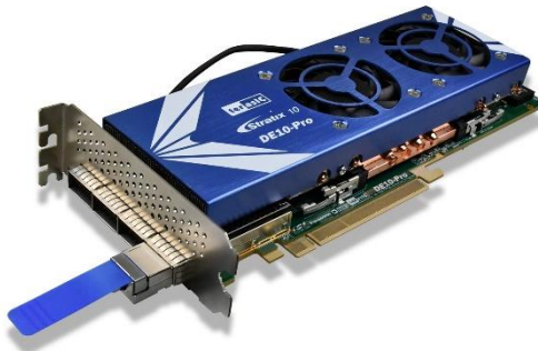
Figure 9-7 Setup QSFP28 loopback fixture
