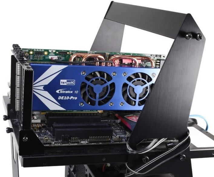
Figure 7-9 FPGA board installation on PC
