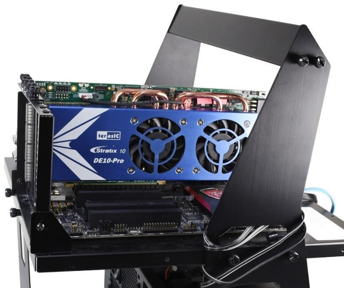
Figure 8-4 FPGA board installation on PC
