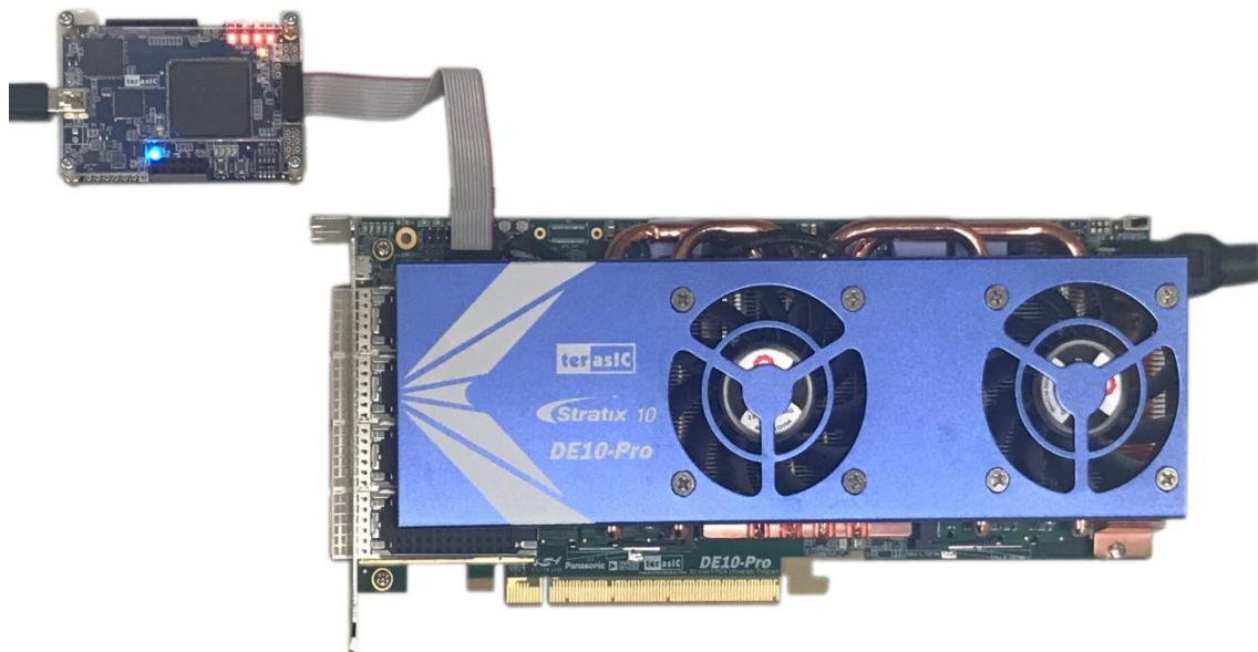
Figure 5-2 Using T-Core board as an USB Blaster II cable
