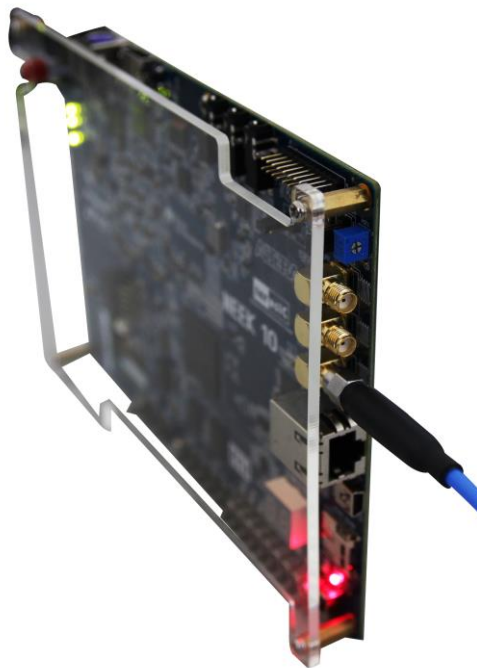
Figure 5-7 Probe DAC SMA OUT from the Oscilloscope
