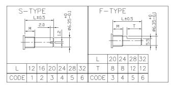
Note 3: Shaft Position (F-Type Shaft) Dashed lines on Type "C" and Type "A" shows position of adjustment slot for S-Type shaft
