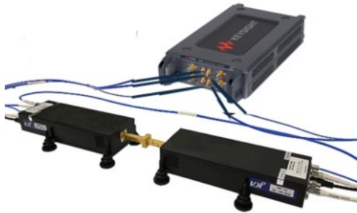
E-band VNA solution using P502xB and N5252AW frequency extenders.
