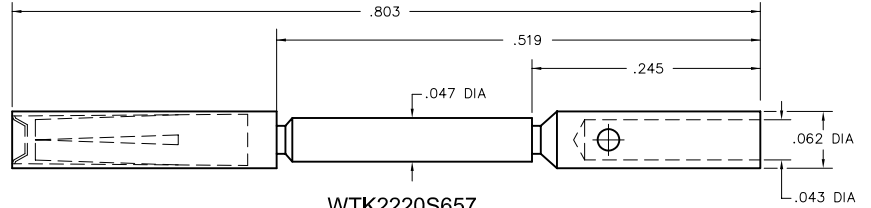
WTK2220S657 SOCKET, CRIMP REMOVABLE, 20 GAGE BARREL
