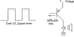
The base current, Ib, should be high enough so that it saturates the collector current of the transistor with the CB load.
