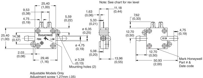
Adjustable Models Only Adjustment screw 1,27mm (,05) Hex socket – clockwise to increase actuation point, counterclockwise to decrease actuation point
