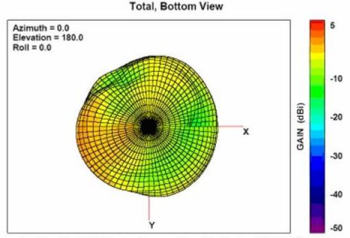
Free-Space Total GAIN, Bottom View, ~~paNodes [2] ~dStartFreqMHz %-0.1f>> MHz
