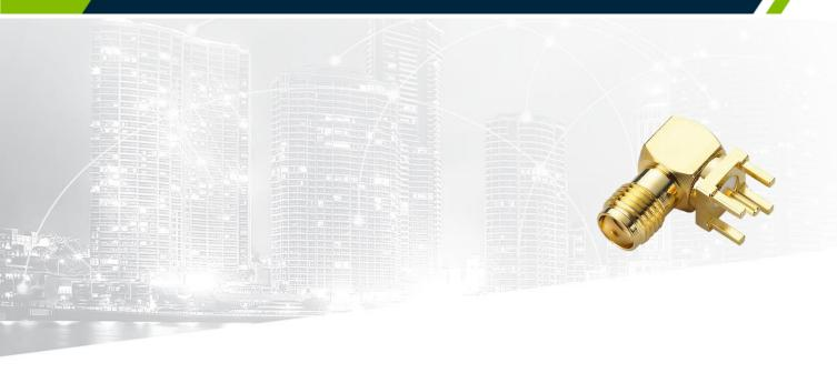
The PCB. SMAFRA.HT connector was designed to be mounted on a PCB. The maximum thickness of PCB that the connector can be used with is 0.4mm. The connector pin is directly soldered onto pads on the PCB. The connector is a standard SMA(F) RA Jack. Taoglas connectors are all RoHS compliant.
