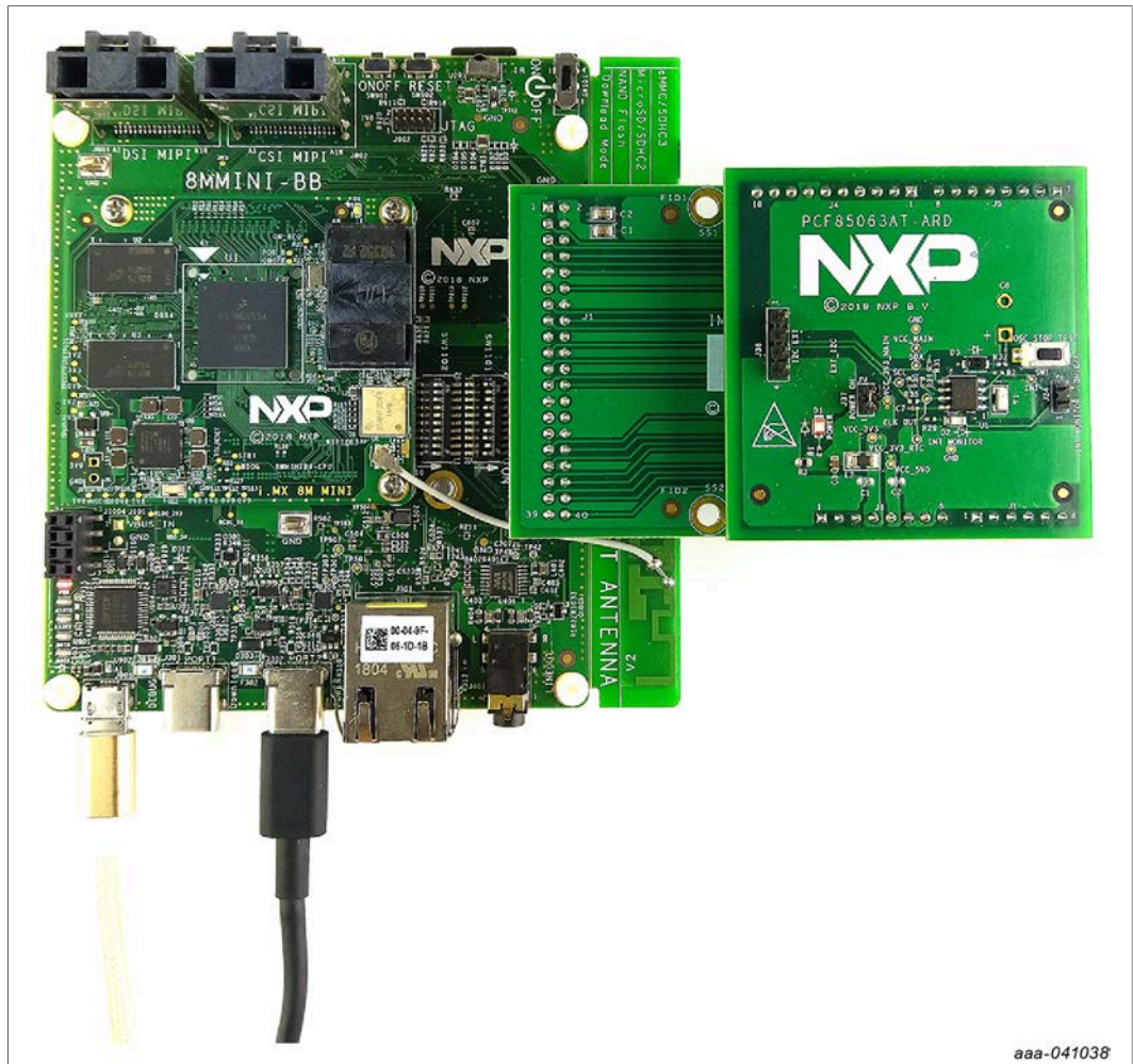
Figure 9. PCF85063AT-ARD daughter board / 8MMINILPD4-EVK board operation
