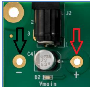
Figure 6 Power via holes
