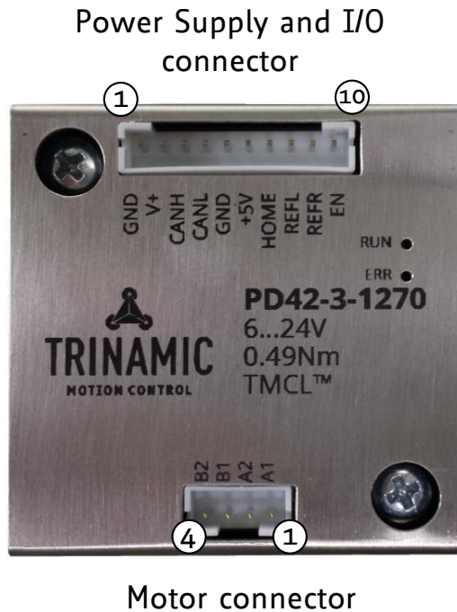
Figure 11: PD42-1270 connectors
