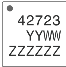
Figure 19 • Package Marking Specifications for PE42723
