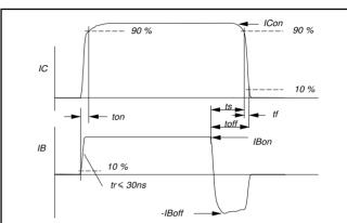
Fig.4. Switching times waveforms with resistive load.
