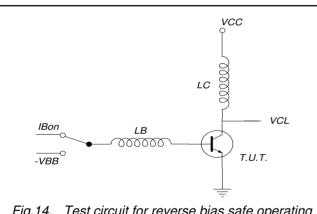
Fig.14. Test circuit for reverse bias safe operating area.
