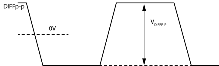
Figure 6-5 Definition of Differential Voltage and Differential Voltage Peak-to-Peak
