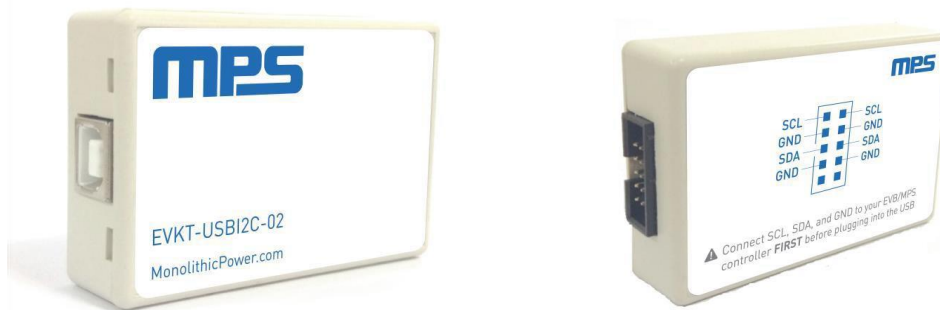
Figure 3: EVKT-USBI2C-02 Communication Interface Device
