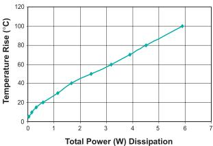
Total Power Dissipation = Copper Loss (W) + Core Loss (W)
