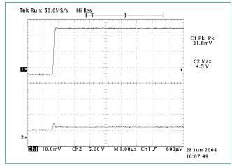
Channel 1: current through LEDs (318 mA) Channel 2: voltage across PLED component (4.5 V)
