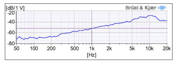
Typical Frequency Response Near-Field vs. Far-Field (2.54cm vs 50cm)
