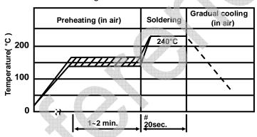
Preheating: 150 +/- 10 °C 1min. to 2 min. Soldering: 240 °C 20sec.
