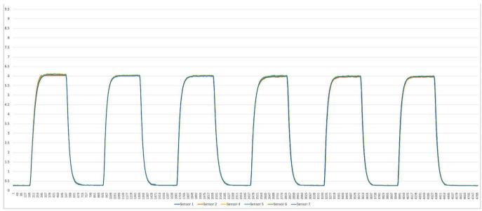
The test results show that the repeatability error range is <20ppb (10ppm  $\pm$  1% of full scale is the normal range);
