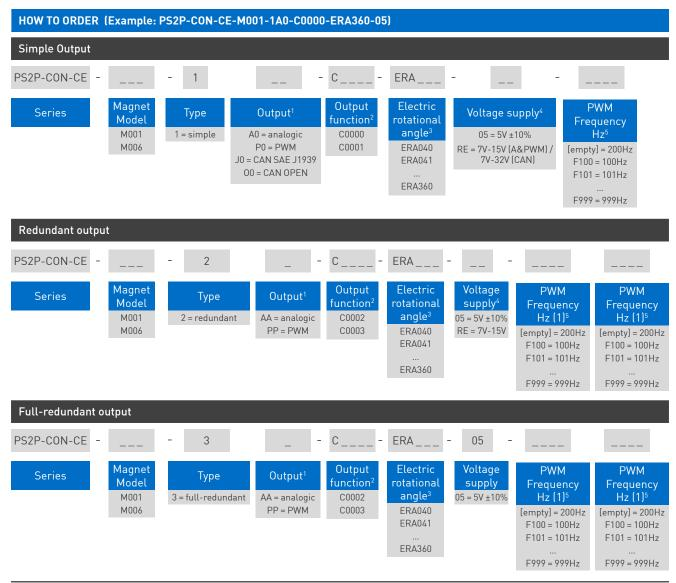
1 The analog output is ratiometric, proportional: - for supply voltage "5V" to input voltage; - for supply voltage "RE" to 5V.
