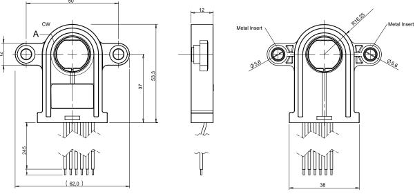
$Sensor\ shown\ above\ is\ the\ 17mm\ version\ with\ the\ rotor\ at\ zero\ position.\ Sensor\ is\ delivered\ at\ random\ position.\ Wires:\ 0.35mm^2\ TXL\ SAE\ J1128$
