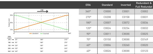
All output functions listed are centered in 180°. Output level from 10% to 90%
