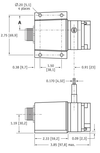
\* tolerance = +.005 -.001 [+.13 -.03] \*\* tolerance = +.005 -.005 [+.13 -.13]
