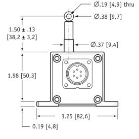
DIMENSIONS ARE IN INCHES [MM] tolerances are 0.03 IN. [0.5 MM] unless otherwise noted.
