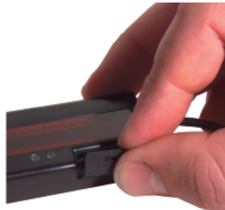
Figure 6. Cover Replacement – Aligning Cover
