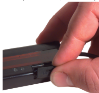
Figure 6. Cover Replacement – Aligning Cover
