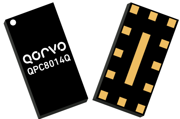
13 Pin 1.1 x 1.9 x 0.44 mm Module Package
