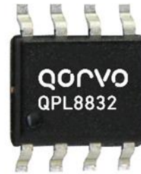
8-Pin SOIC Package
