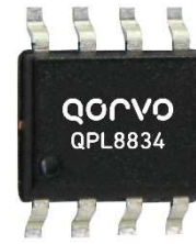
8-Pin SOIC Package
