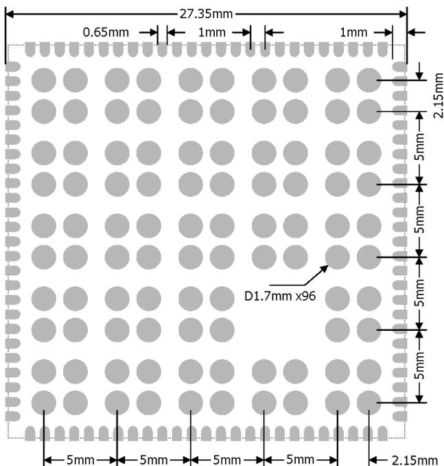
Aperture size of the stencil is 1:1 with the pad size. Four 1.7mm diameter bumps are used for each of the 4.3mm square GND pads sections giving a 50% solder paste padding. The lower component settling with this ensures that the pads at the edge are always soldered even at vertical misalignment by distortion or warping.
