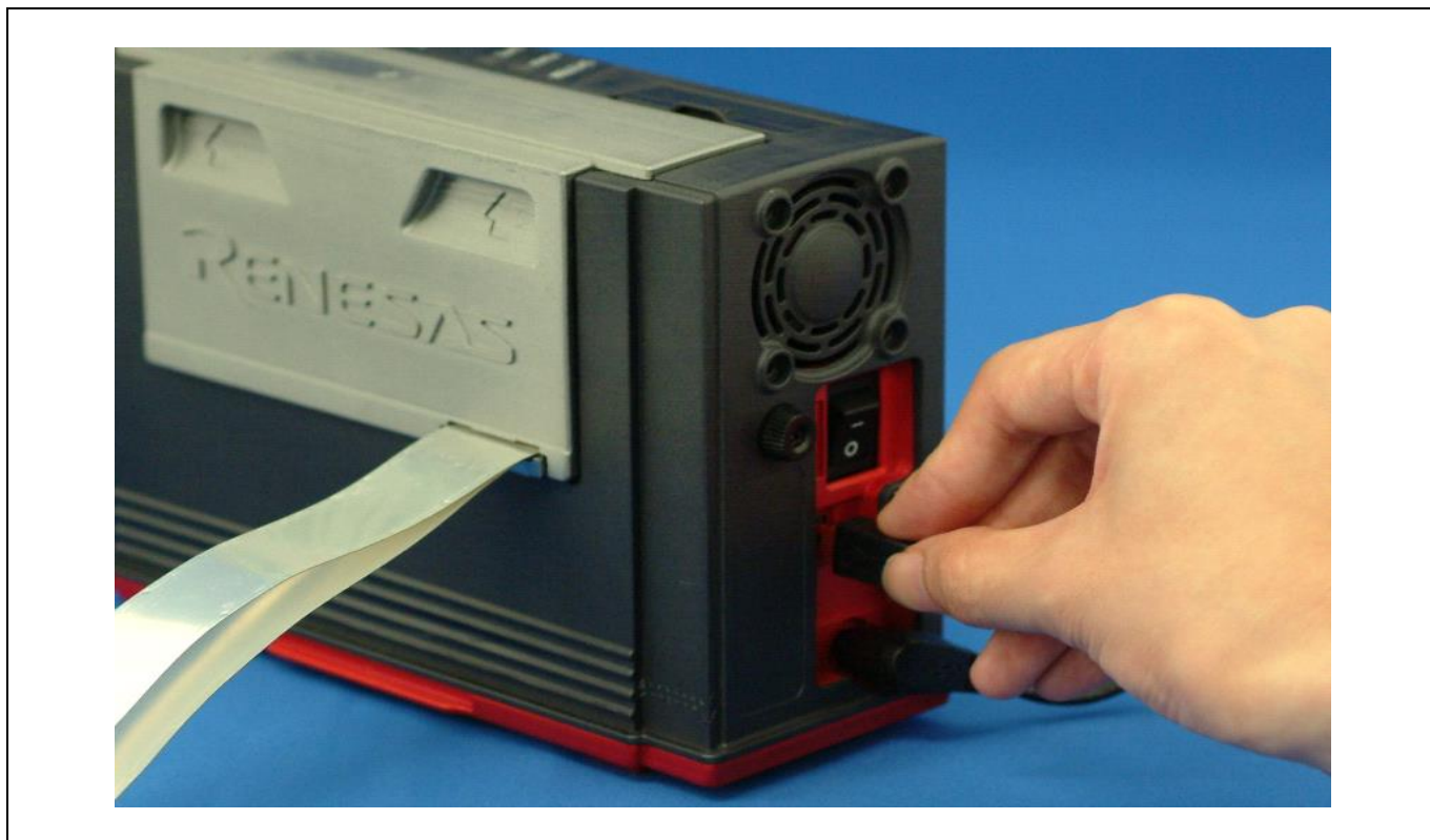
Figure 2.4 Connecting the host machine
