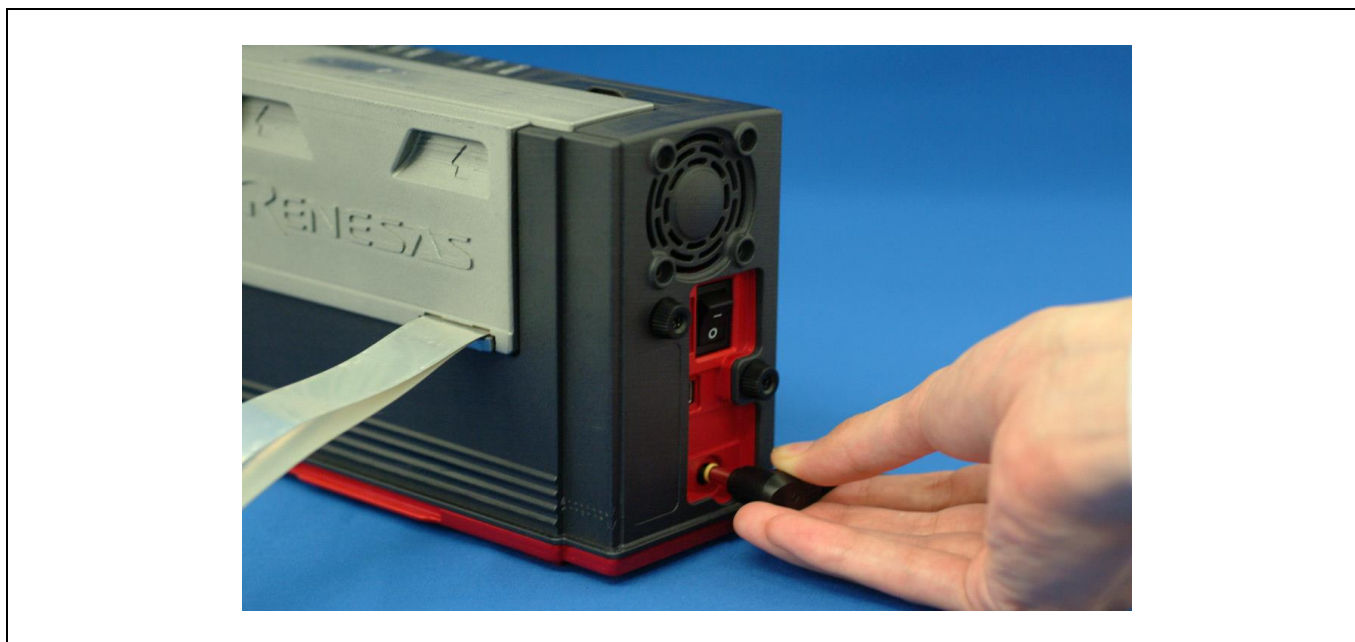
Figure 2.5 Connecting the emulator power supply
