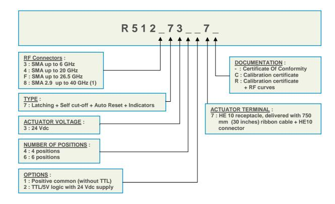
(1) Connector SMA2.9 is equivalent to "K Connector®", registered trademark of Anritsu
