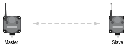
Figure 2. Simple point to point network
