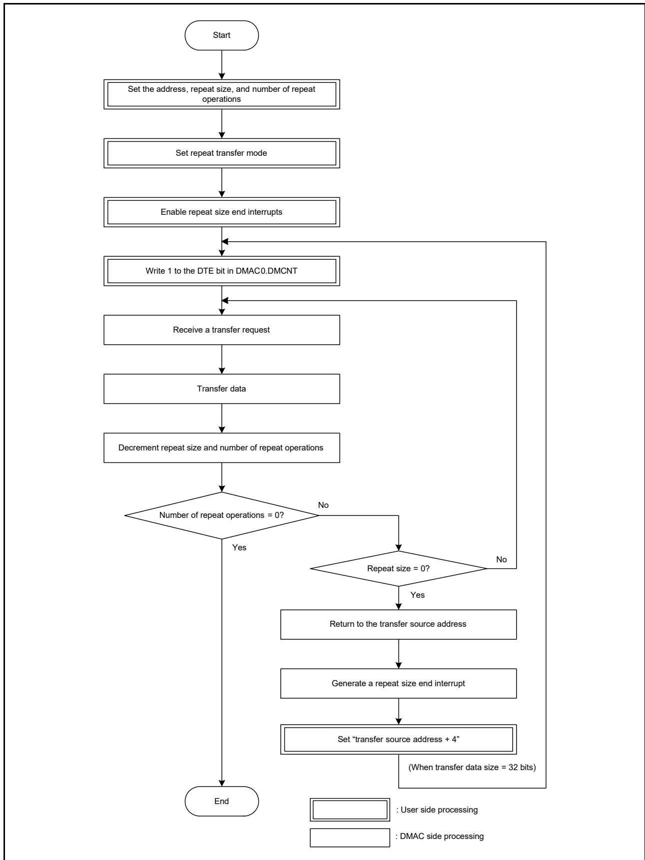
Figure 16.9 XY conversion flow using offset addition in repeat transfer mode
