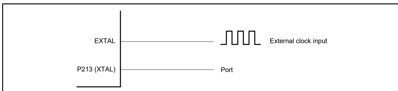
Figure 9.8 Equivalent circuit for external clock
