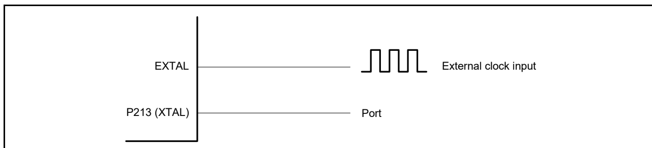
Figure 9.8 Equivalent circuit for external clock
