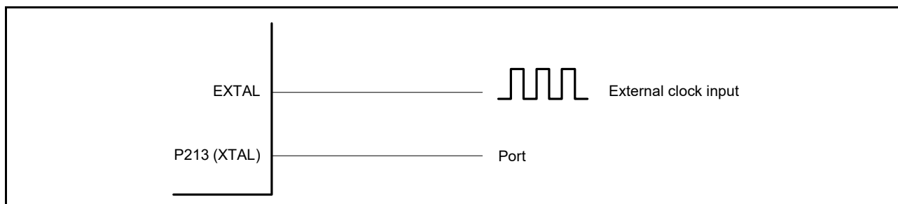
Figure 9.8 Equivalent circuit for external clock
