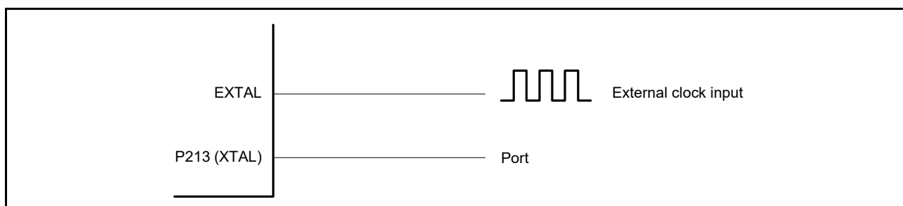
Figure 9.8 Equivalent circuit for external clock
